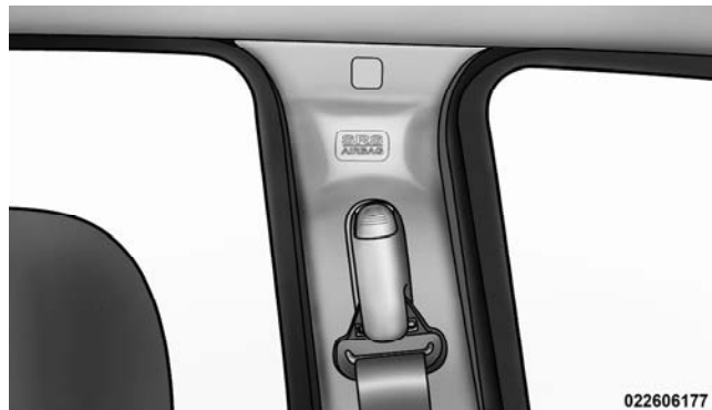
Supplemental Side Airbag Inflatable Curtain (SABIC) Location
