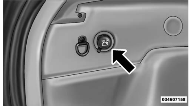
Rear Power Outlet
