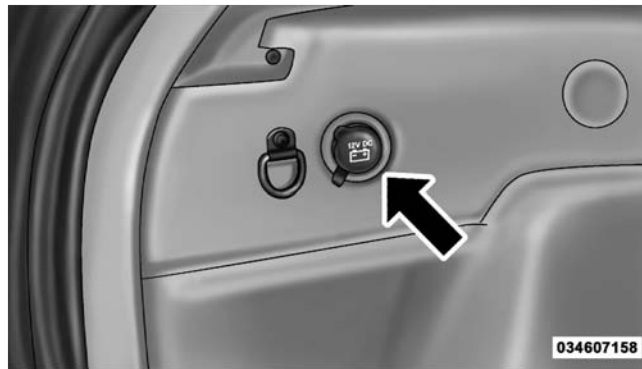
Rear Power Outlet
