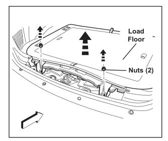
**3)** Remove load floor (two 10mm nuts, 10mm socket and wrench).
