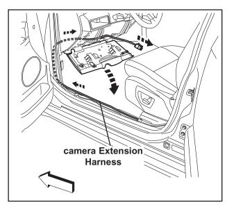
**23)** Lower knee bolster and route Camera Extension Harness as shown (hook/pry tool).
