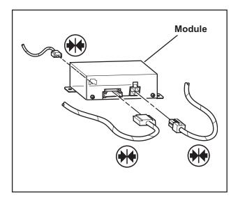
14) Connect harness connectors from monitor, t-harness and Camera Extension Harness to Module (Item 9).
