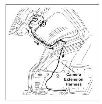
**11)** Route camera extenstion harness as shown into roof cavity, tie strap as needed.
