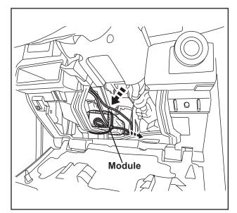
**16)** Secure module to knee bolster brace to the left of the steering wheel using Tie Straps (Item 11).
