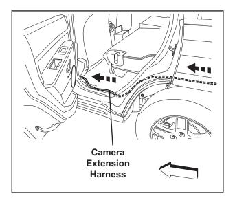
**18)** Route Camera Extension Harness forward as shown tucking harness under the edge of the carpet.
