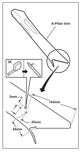
**10)** Mark initial drill point as shown, from initial drill point, mark additional drill points as shown.
