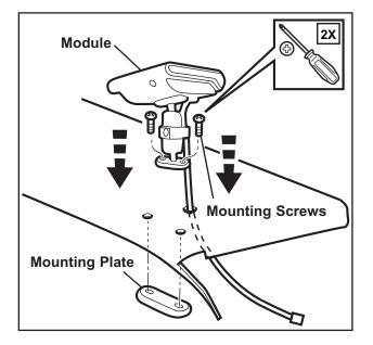
**12)** Route harness from monitor (item 8) through A-pillar as shown. Mount monitor to A-pillar using screws (item 13) with philips head screw driver to mounting plate (item 12).
