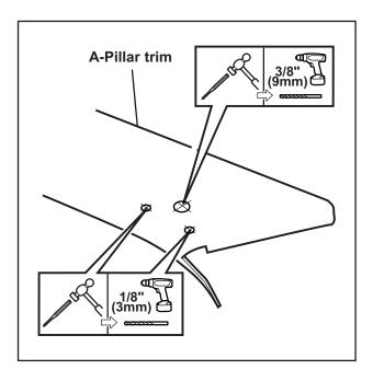
**11)** Punch and drill holes as shown, (1/8" drill bit for lower holes, 3/8" drill bit for upper hole).
