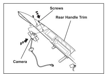
Install Camera (Item 2) to rear trim handle Using two Screws (Item 3) and Nuts (Item 4) (phillps screwdriver).
