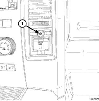
Using a trim stick C-4755 or equivalent, disengage the retainer clips that secure the trim ring to the floor console.
