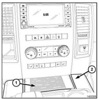
3. Using a trim stick C-4755 or equivalent, disengage the retaine clips that secure the power outlet trim bezel (1) to the center bezel (2).
