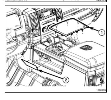
clips that secure the shifter bezel to the floor console
