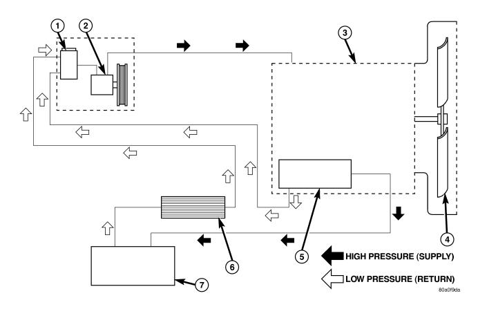
Fig. 2 HYDRAULIC FAN FLUID FLOW CIRCUIT
