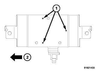
Fig. 1 REVISED SDAR MOUNTING HOLE LOCATIONS
