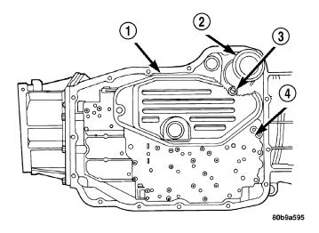
Fig. 2 Transmission Filters - 4X4 Shown
